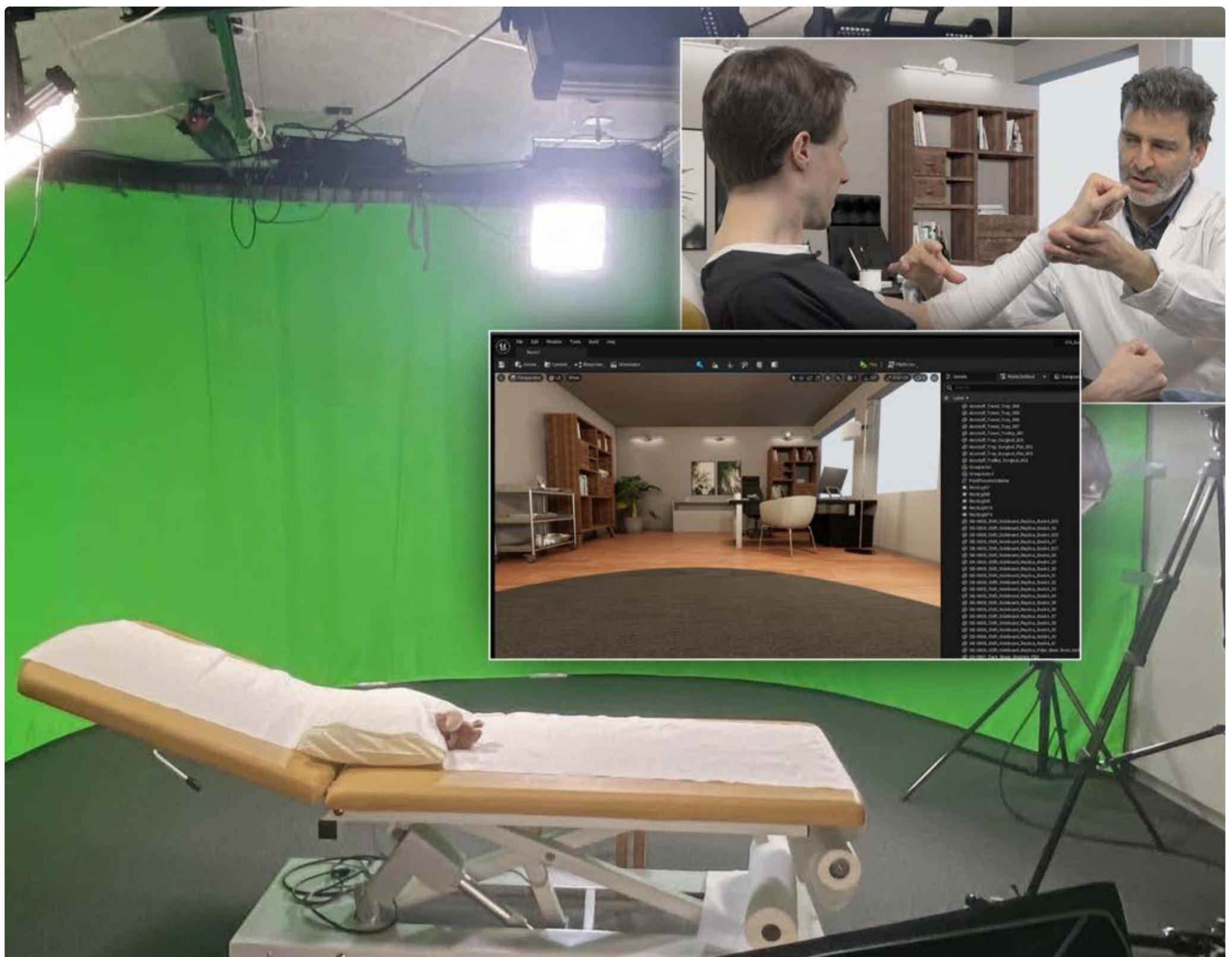
ecording in Greenscreen Setup and the artificial background plate in Game Engine are composed to a final result
